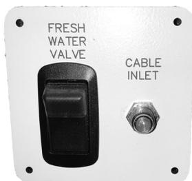
The touring coach is also pre-wired for a portable satellite antenna. The exterior inlet is located in the roadside rear compartment of the touring coach and is labeled for your convenience. The interior pre-wire is located in the front overhead roof locker.
