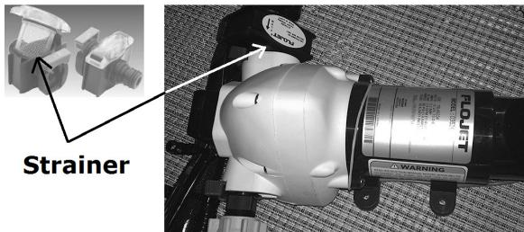
To clean the strainer screen: With the clear plastic at the top, press on the sides of the strainer releasing the tabs holding the clear plastic top in place, hold the sides in, and pull straight up on the clear plastic top to remove the screen assembly. Rinse all debris from the screen. Replace the screen assembly by aligning the screen in the seating groves and pressing gently down until tabs catch and hold the clear plastic top in place.
