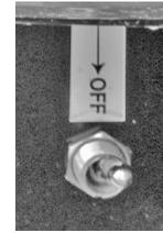
A remote switch for shutting off the gas to all appliances is located in the curbside rear utility compartment. The switch activates an electric solenoid which opens and closes, shutting the gas off at the tank. This switch should be turned off during the filling of the LPG tank.
