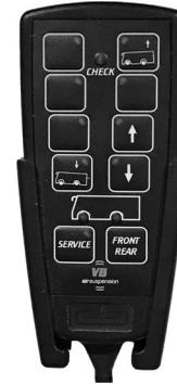
A remote, located on the B-pillar next to the drivers seat, can be used to manually adjust the air suspension. To manually adjust, while parked set the emergency brake. With the engine running, press and hold the up or down arrows to raise or lower the rear of the van to the desired level. A short press of the up or down buttons will raise or lower the coach to its highest or lowest position.
