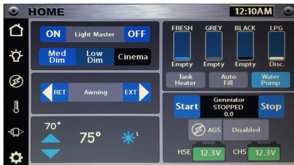
The “Home” screen of the Multiplex Systems main control panel displays the fluid levels of the Black Water, Grey Water, Fresh Water tanks, and the LP gas tanks. The panel also shows the voltage status of the main (chassis) and the auxiliary (house) batteries.
