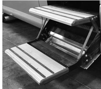
The curbside door has a folding double step with auto retract, step out warning buzzer, and a lock extended switch located just inside the door. Please read, understand, and instruct passengers of the following operational and safety information pertaining to the step.
