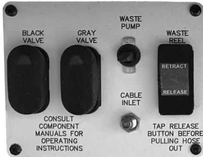
1. Remove the high pressure waste hose by opening the hose reel compartment door and momentarily pressing the “release” switch. Once released the hose can be manually pulled out. Secure the hose at the disposal facility inlet using the threaded or rubber adaptor and open the drip proof valve on the end of the hose.
