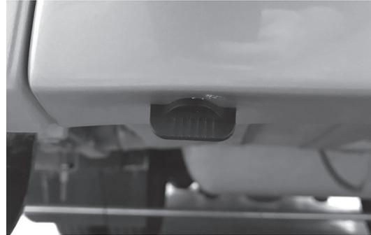
2. Rotate each wing nut 1/4 turn, pull down and remove.
