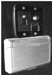
An exterior receptacle is located in the curbside utility compartment between the wheels and step. Also in this compartment is the exterior cable hook-up, HDMI inlet, and USB ports. A motion sensor light has been installed for your convenience. The light can be manually switched off if needed, however, if switched off the motion sensor will not function.
