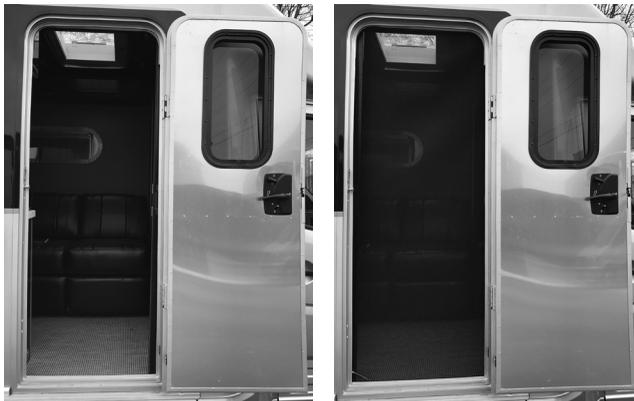
The screen door is secured to the threshold of the main door and can be operated independently by sliding and latching it via a magnet catch. This innovated door takes a fresh approach to maximizing fresh air and your view while offering a smooth and steady screen operation.
